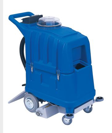
Running under 60 dB, the AV 12QX is an excellent choice for any 24 hour facility, especially in the hospitality and healthcare industries. The AV12QX is constructed of polyethylene and features a 130 psi pump providing a flow rate up to 1.2 gpm. The powerful 1.8 hp, three-stage vacuum motor provides 135-inch water lift and 95 cfm of airflow. The spring-loaded vacuum shoe is adjustable, ensuring consistent pressure and pick up on different carpet thicknesses and uneven floors.
