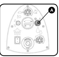
Insert the Ignition key and switch the machine on. (Fig. A)
