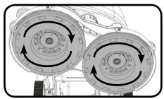
$2\times370$ mm Brush or a  $2\times360$ mm Pad on the TGB 8572. Featuring the Nulock brush system. The brush is simply pushed and twisted to lock, making fitting and removal a simple process.
