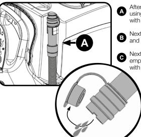
After use, empty waste water tank using emptying hose and flush out with clean water.
