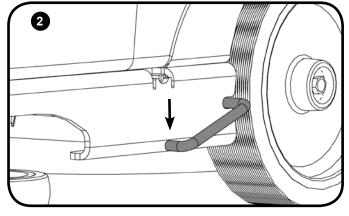
The machine is equipped with a free-wheel function that will enable the operator to move the machine manually if required.
