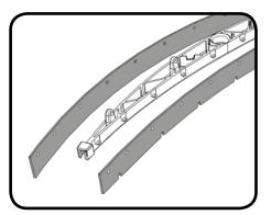
Periodically the floor tool blades should be examined and checked for wear and damage. The blade removal is easy. Simply start by removing the four retaining pins, turn the floor tool over and separate the blade carrier from the body. Peel away the blades from their locating lugs and examine or renew as required. Replacement is a reversal of the removal process.
