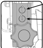
LH Bias: If the machine pulls to the right, turn the knob clockwise to apply left hand bias to the brush deck.
