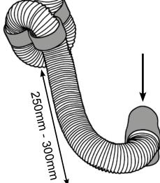
Refit vacuum hose to the Floor tool when finished.
