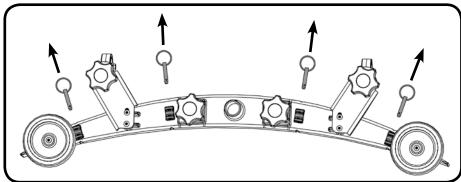
To clean the floor tool, remove securing-pin and pull-free from the holder. Rinse the floor tool assembly with clean water and refit.
