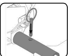
Fit the floor tool and retain using the detent pin.
