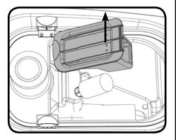
Located under the top tank at the front of the machine is a clean water filter.
