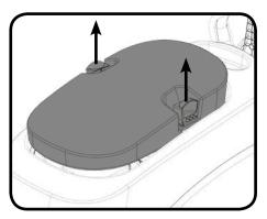
Whilst pressing in the top tank hood toggles, remove the hood.
