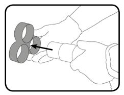
NOTE: DO NOT push the vacuum hose onto the floor tool with the floor tool in the raised position.
