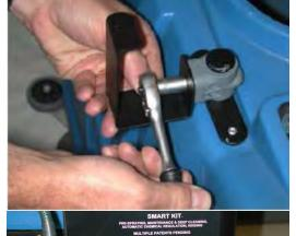
With hose holder and 10mm bolt provided, attach as shown to the left.
