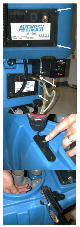
Remove two screws (top right and bottom right) from machine plate as shown.
